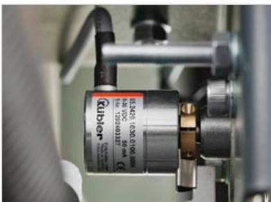
Direct measurement via rotary transducer flanged to the spindle
