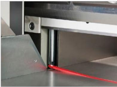
A cutting stick ejector eases and abbreviates the knife change
