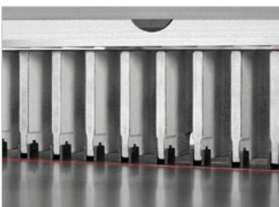
Backgauge rakes with plastic gliders treat the table surface with care
