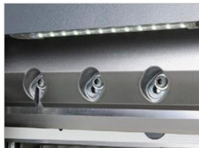
LED cutting-line indicators ensure optimum illumination, even when lighting is poor. The indicator can be clearly seen on many materials.
